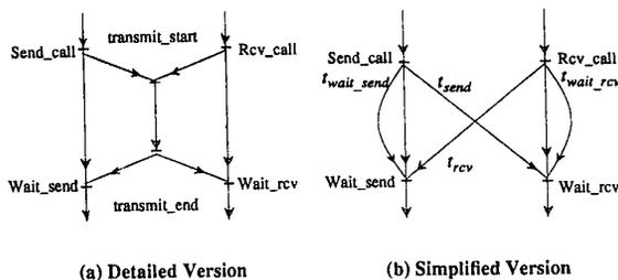
Figure 2: Construction of Simple Program Activity Graph
