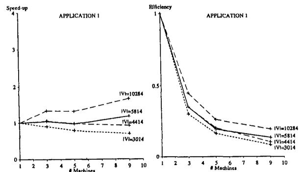
Fig. 3: Speed-up of Distributed Algorithm
