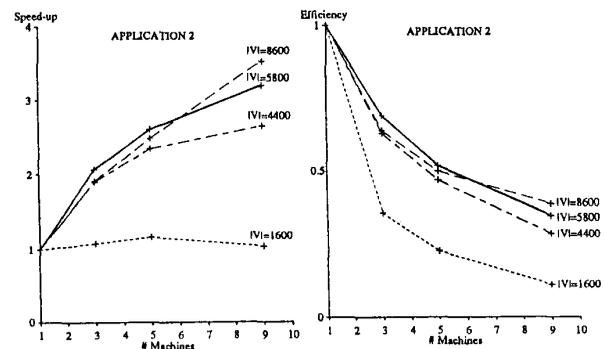
Fig. 5: Speed-up of Distributed Algorithm
