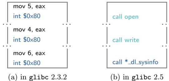
**Figure 1: An example of function inlining in the wrapper function `sethostid`.**
