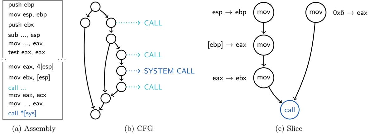
**Figure 2: The semantic descriptor generation process.** From the raw instructions of the function (a), we generate the control flow graph (b) and identify all **system calls** and **wrapper function calls**. We slice (c) backwards over the instructions in the CFG to determine the system call number and any arguments that can be concretely identified using symbolic evaluation. The system calls and concrete parameter values forms the semantic descriptor for this function.
