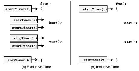
Figure 1 Timing instrumentation for function foo.
